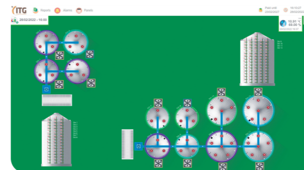
ITG® Cloud - Multi-functional, specialized software for temperature monitoring, analysis, and ventilation process control with remote access through a cloud-based platform.
